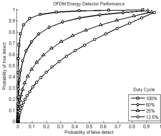
Fig. 8. ROC curve for wideband energy detector for OFDM signals with 10 dB SNR and 100%, 50%, 25%, and 12.5% duty cycles.
