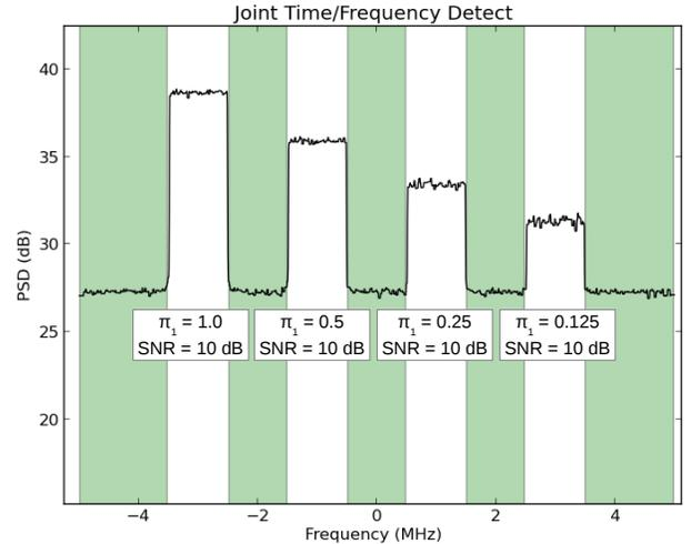
Fig. 6. Results of joint time-frequency detector for OFDM signals with 10 dB SNR and 100%, 50%, 25%, and 12.5% duty cycles.
