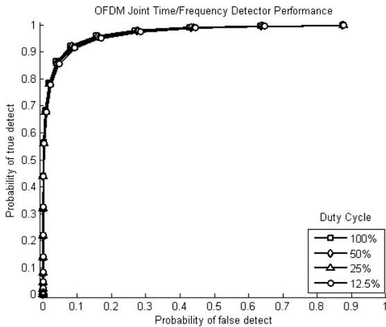
Fig. 10. ROC curve for joint time/frequency detector for OFDM signals with 10 dB SNR and 100%, 50%, 25%, and 12.5% duty cycles.
