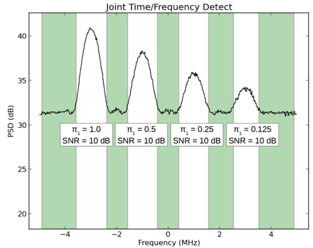
Fig. 7. Results of joint time-frequency detector for GMSK signals with 10 dB SNR and 100%, 50%, 25%, and 12.5% duty cycles.
