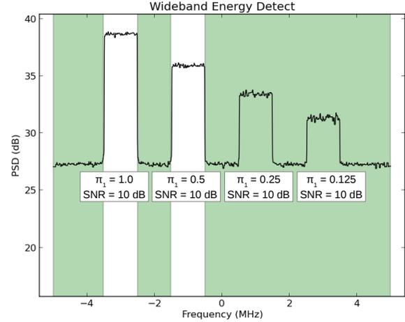
Fig. 1. Results of a wideband energy detector for OFDM signals with 10 dB SNR and 100%, 50%, 25%, and 12.5% duty cycles.
