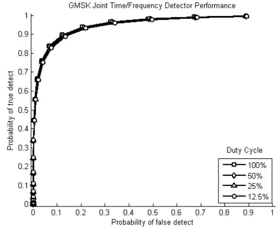
Fig. 11. ROC curve for joint time/frequency detector for GMSK signals with 10 dB SNR and 100%, 50%, 25%, and 12.5% duty cycles.
