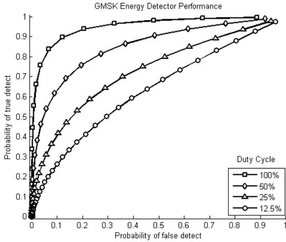
Fig. 9. ROC curve for wideband energy detector for GMSK signals with 10 dB SNR and 100%, 50%, 25%, and 12.5% duty cycles.
