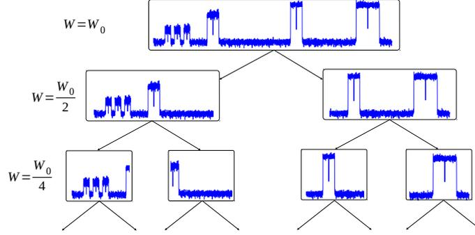
Fig. 5. A spectrum band with center frequency  $f_{c0}$  and bandwidth  $W_0$  organized into a balanced binary tree.
